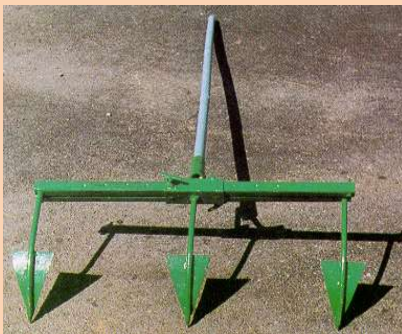
Fig: Adjustable Row Marker
