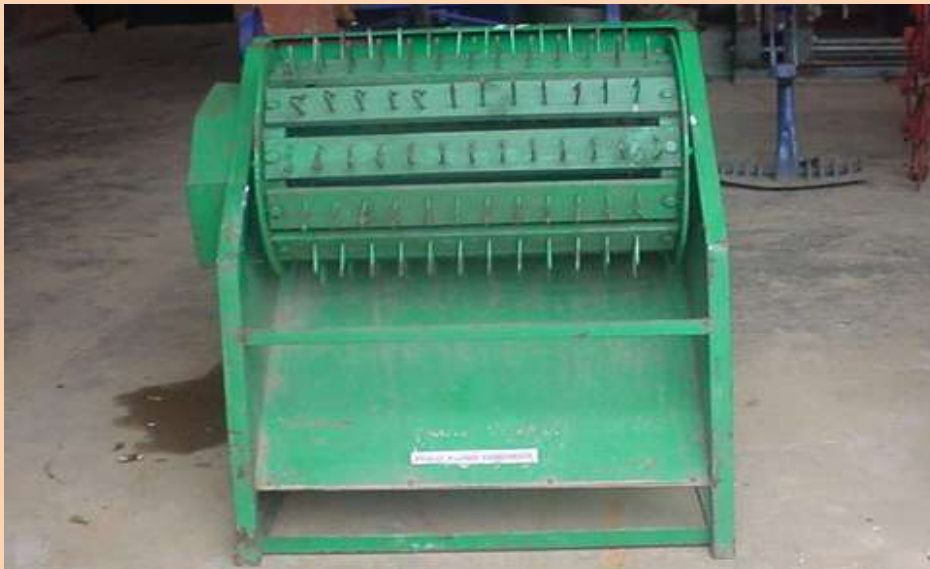
Fig : Paddy Operated Paddy Thresher
